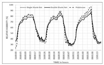
**Fig. 7:** Relative humidity variation inside the three housings (with seeded soil pots)
