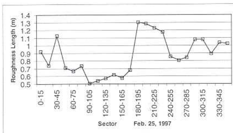
Fig.11: Variation of roughness length derived using maximum IRS-1C/WiFS NDVI within 15^\circ sectors.
