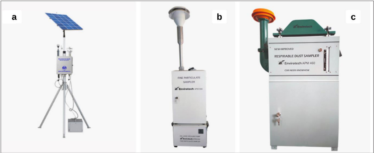
Fig. 2: Ambient air quality monitoring: (a) Sensor-based mini ambient air quality monitoring system (Mini AAQMS), (b) APM 550 fine particulate sampler, and (c) APM 460 respirable dust sampler
