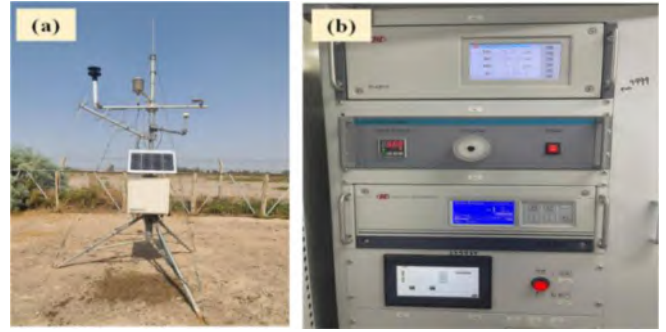
Fig. 2: Dataset sources, (a) 110-WS-25 standard weather station, (b) PS7400 system.
