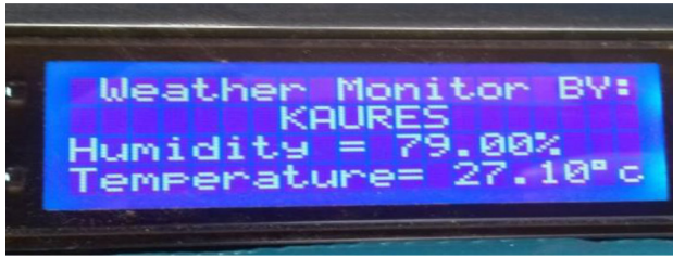
Fig. 3: Sample of the recording of the humidity and temperature on an LCD monitor
