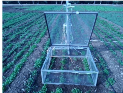
Fig. 2: Measurement of coriander ET_c in field by PACCC
