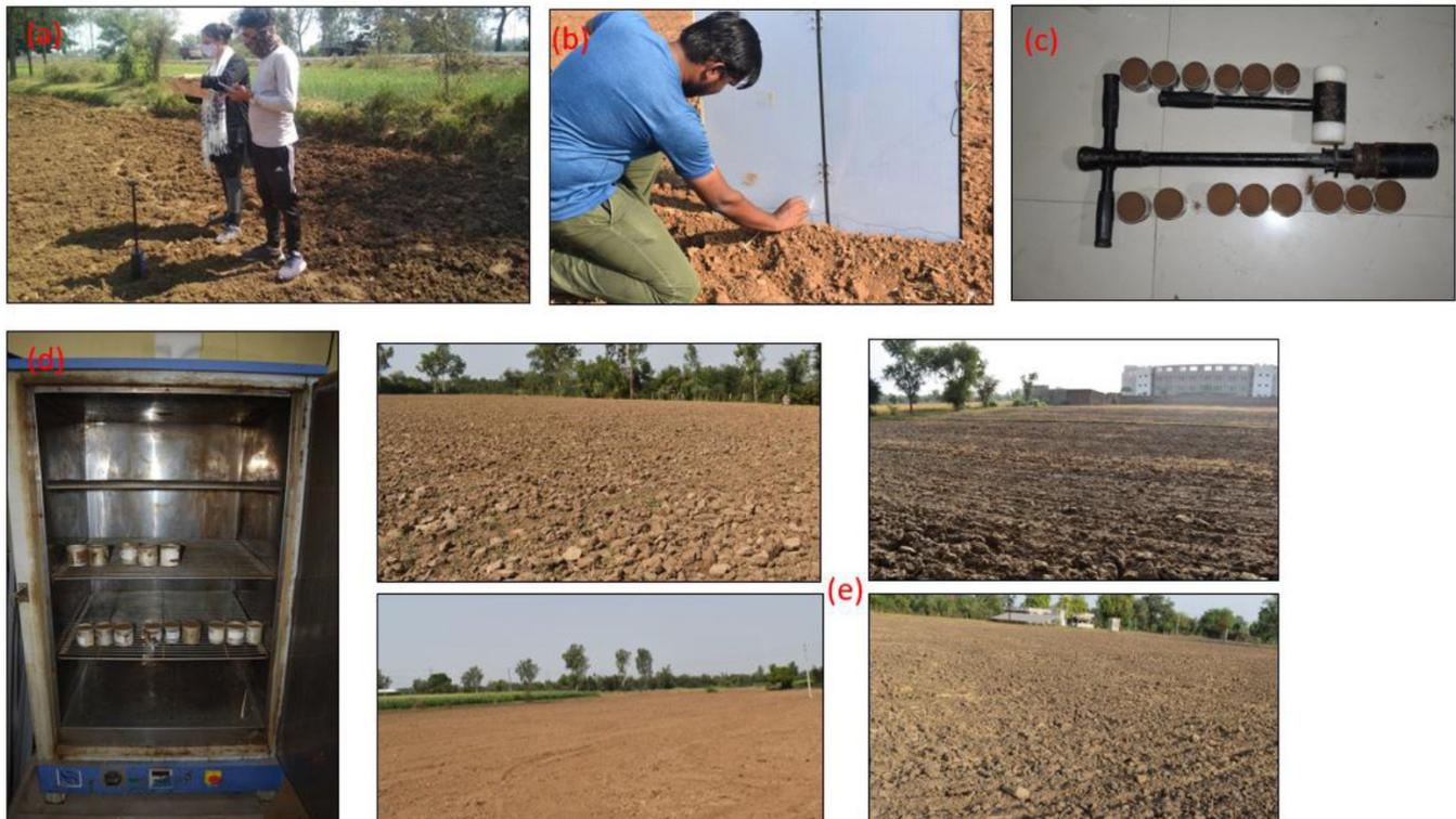
**Fig. 2:** (a) Soil Moisture measurement using HydraGo Probe (b) RMS height measurement using roughness plate (c) Gravimetric measurements using core sampler with auger (d) Oven drying of the samples (e) Various soil conditions during field visit.
