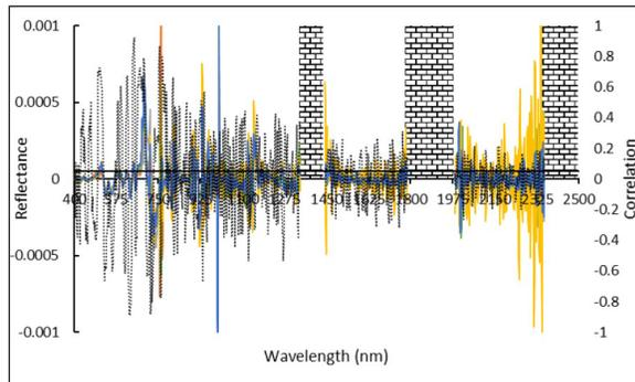
**Fig. 2c:** 2<sup>nd</sup> order derivative spectral reflectance of different severity grades and their correlation
